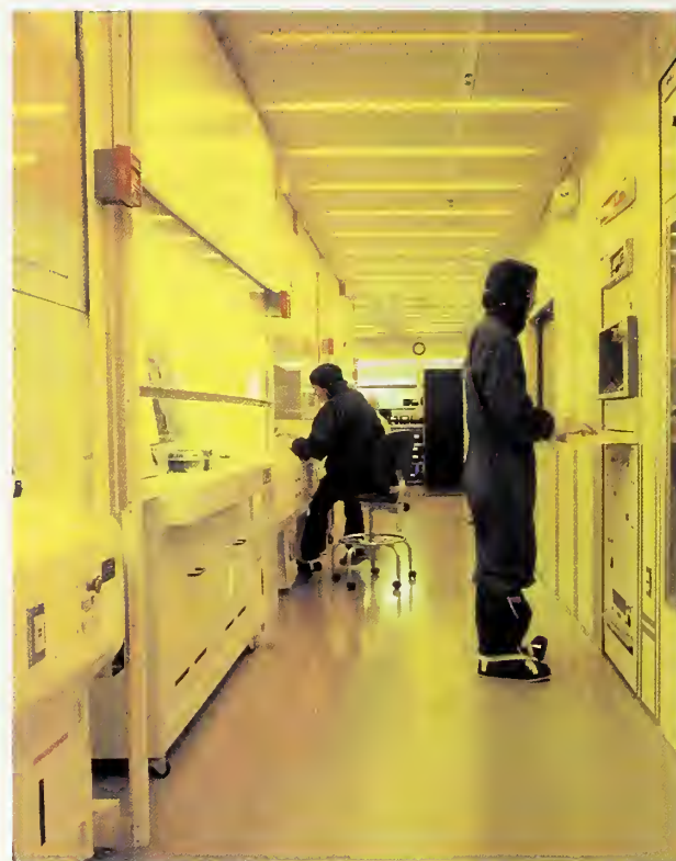
Figure 2. View of clean room lithography bay with digital pattern generator and wafer stepper recessed into the wall on the right and wet processing on the left. Optical lithography produces linewidths smaller than 500 nm and is often combined with electron beam lithography for structures as small as a few tens of nm.
